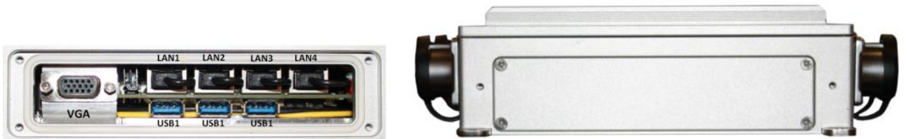
NANO-BOX i7-8665 internal connectors protected from IP65 aluminum door
